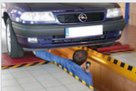
Two test plates at ground level integrated in the base
