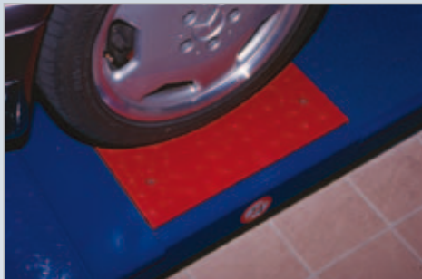
PMS, type 3/X can be integrated in an installation pit or in a lift, e.g. DUO. We recommend the other types for the installation pit.
