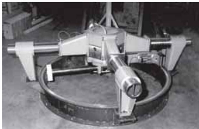
*Originally designed to machine eight-foot diameter stainless steel heat exchanger flanges in a nuclear fuel reprocessing plant, the FF8000 Flange Facer has an OD-mount feature, shown here.*
