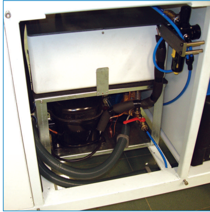
Built-in refrigeration system
