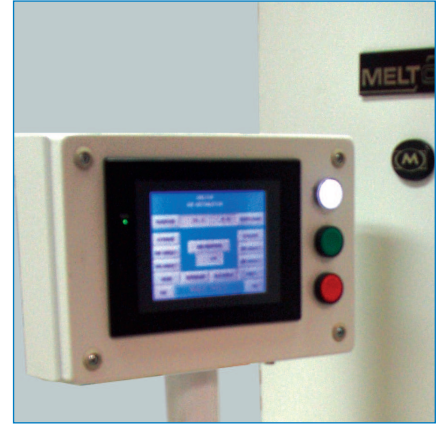
Touch-Screen panel for operation
