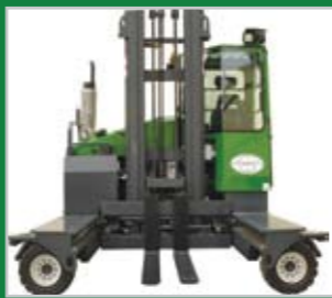
Integrated Hydraulic Fork Positioner
