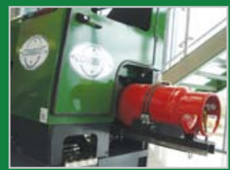
Sliding LP Gas Tank
