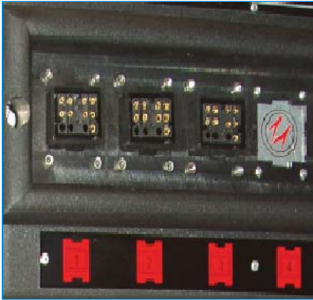
Up to 4 hose-gun connections.
