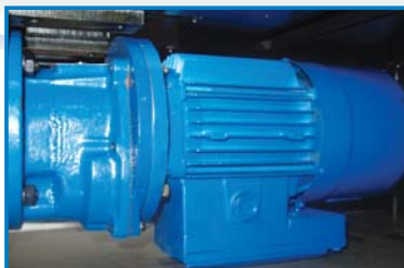
Variable speed AC motor with VFD integrated control
