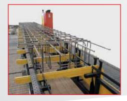
The positioning of the stirrups allows the operator to build cages in absolute safety, while preventing the excessive strain caused by lifting and supporting longitudinal bars.
