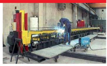
• Extension for support of cages up to 2400 mm • Additional welding trolley. (OPTIONAL) in width. (OPTIONAL)
