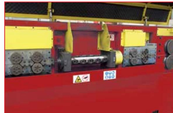
**Two infeed units** drive properly the wire, guaranteeing **constant speed and straightening quality**, making it particularly **suited for small diameters**. Based on the different lengths and diameters can be possible to work with setting of **different speeds**.
