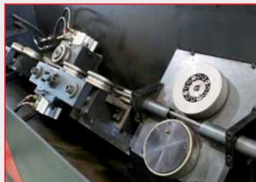
The insertion and straightening unit has an independent infeed that allows a **constant control of the wire speed**, originated by the hyperbolic rotor, based on the different diameters. An optimal quality of straightening is thus achieved.
