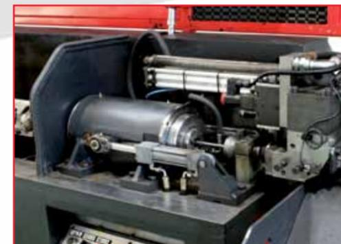
The flying shear cut to length the wire while is moving ensuring **high speed performances** and the **respect of the measurement tolerances**.
