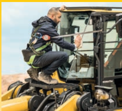
Front cleaning step for safe and easy access to the front window
