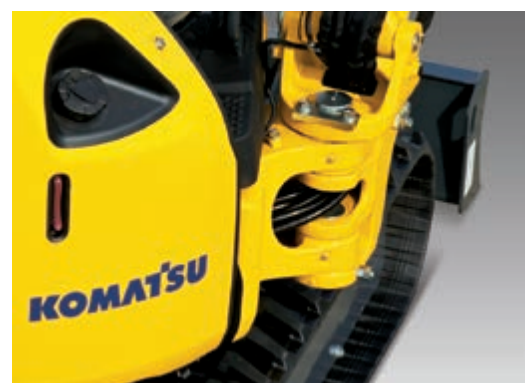
The swing cylinder is now relocated to the left side of the excavator to minimise protrusion. The operator doesn't have to worry about it when working near a wall.
