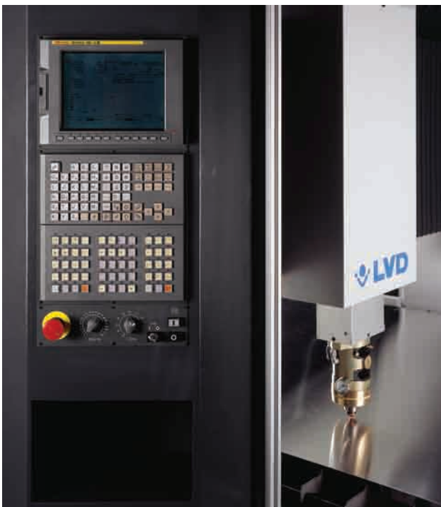
Integrated laser source and control
