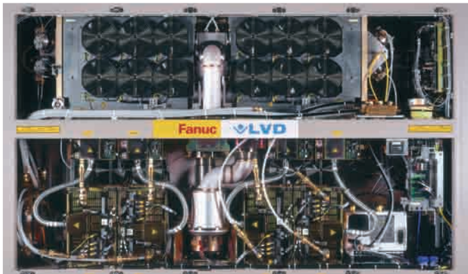
Fast axial flow CO 2 laser
