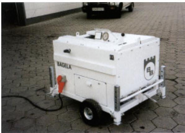
KTW 1000 with electric motor and supporting jacks
