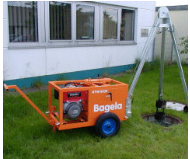
KTW 1005 with wheels, tow bar and triple beam (extra accessories) for sewerage cleaning jobs.
