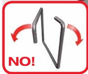
The twisting of the wire during the pulling phase creates open stirrups.
