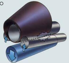
contrary, guiding the shorter edge of the plate (at the tight diameter of the cone) to slightly rotate according with the cone geometry, slows down the feeding of its shorter development. Side rolls must be tilted to form the cone at its right geometry. Davi 4 roll have, as standard feature, the electronic bottom clamping and side rolls tilting, up to a level substantial higher than the competition (Davi exclusive and benefit).
