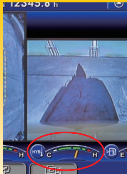
Hybrid system temperature gauge
