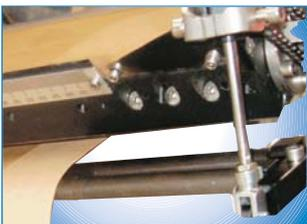
Possibility of roller bracket and position guide. Lip pressure control designed for fragil material works.
