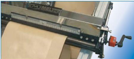
Easy and precise coating width, side or centered, hand adjustment. Regulation crank position available at right or left.
