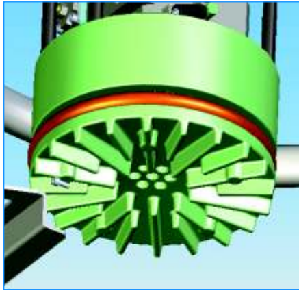
Finned, flat and new axial platens for maximum melting capacity
