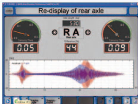
Significant representation of defective axle damping (example)
