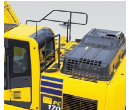
Hand rails and anti-slip plates
