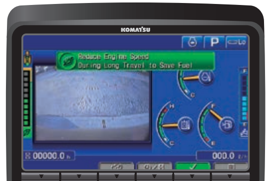
Improved monitoring system with rear view camera image on the default screen. Eco gauge, eco guidance, fuel consumption gauge and adjustable idle shut-down help to further reduce consumption.
