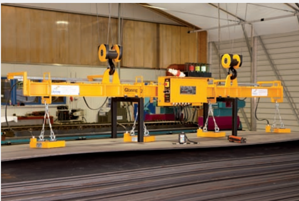
EPM - Magnet-spreader beam M 750-4 single-row, 4 m, lifting capacity 3 t, modules adjustable For lifting of sheets up to max. 6000x2000x4-25 mm 2-circle- control with remote control and tip off function
