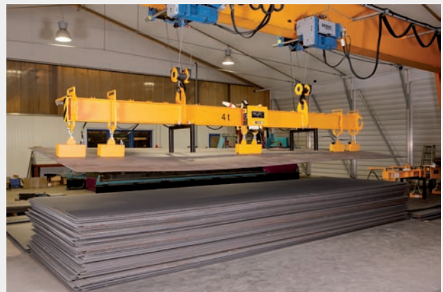
EPM - Magnet-spreader beam 5190-5 Bi-Pol single-row, 5,5 m, lifting capacity 4 t, modules adjustable For lifting of profiles 1 - 10 m, 2-circle-control with remote control and tip off function
